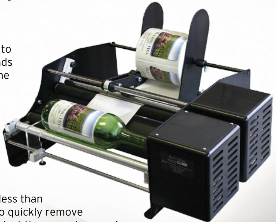
Most wine bottles are labeled in less than five seconds, enabling the user to quickly remove the bottle and insert another to start the procedure again. After a rhythm is established, bottles can be labeled very quickly.
